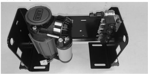
4. CKMA Compressor with ARB LINX PRV, Compressor Switch and quick connect coupling
