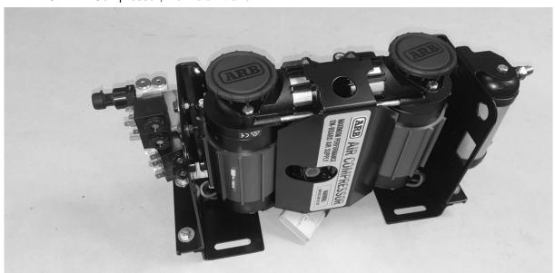
8. CKMTA Compressor, manifold kit ,ARB LINX PRV, Compressor Switch and quick connect coupling
