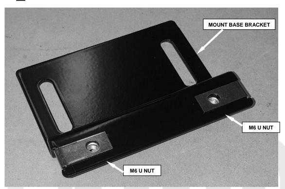
Attach the mount base brackets to the compressor mount bracket using 4 X M6 X 20 HXHD bolts and 4 X M6 X 20 X 1.6mm flat washers, do not fully tighten at this stage. Note the orientation of the mount brackets is determined by the fitting location and the suitability of the mounting surface. The photos below show examples of combinations for fitting the mounting brackets.
