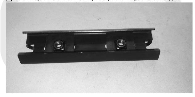
With the aid of an assistant install each clamp plate as shown. If there is a valley, install packers ensuring that the M8 X 35 HXHD bolt passes through each of the packers. The height of the packer should be slightly less that the depth of the valley to ensure a tight joint is achieved.
